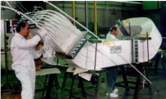
Fig. 13: Saddle-shaped superconducting coil
